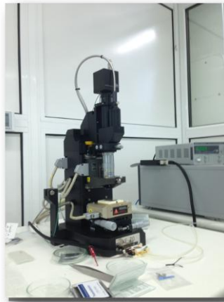
Fig. 2. AFM - XE70 Multifunctional
