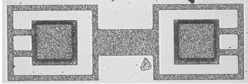
$$\text{Rigiditatea micromembranei: } \delta_{1z} = \frac{F}{3} \left[ K_{b_{cs}} l_1^3 + K_b (l_{13}^3 - l_1^3 + 3l_{13}^2 l_5 - 3l_{13} l_5^2 + l_5^3) + K_t 3(l_1^2 l_2 + l_{13}^2 l_4) \right] - \frac{M_0}{2} \left[ K_{b_{cs}} l_1^2 + K_b (l_{13}^2 - l_1^2 + 2l_{13} l_5 - l_5^2) + K_t 2(l_1 l_2 + l_{13} l_4) \right]$$
